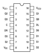
Pin assignment is for Dual-in-Line Package.
