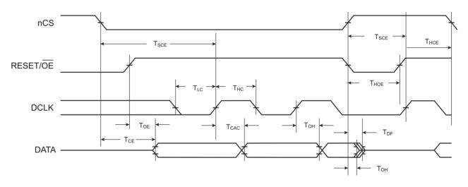
Figure 10-2. AC Waveforms when Cascading
