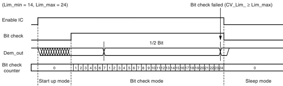
Figure 5-5 on page 16 to Figure 5-7 illustrate the bit check for the default bit check limits  $Lim\_min = 14$  and  $Lim\_max = 24$ . When the IC is enabled, the signal processing circuits are enabled during  $T_{Startup}$ . The output of the ASK/FSK demodulator (Dem\_out) is undefined during that period. When the bit check becomes active, the bit check counter is clocked with the cycle  $T_{XClk}$ .
