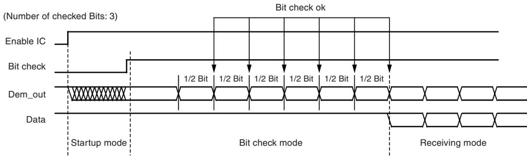
**Figure 5-5.** Timing Diagram During Bit Check
