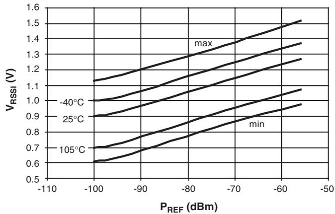
If  $R_{Sense}$  is connected to  $V_S$ , the receiver operates at a lower sensitivity. The reduced sensitivity is defined by the value of  $R_{Sense}$ , the maximum sensitivity by the signal-to-noise ratio of the LNA input. The reduced sensitivity is dependent on the signal strength at the output of the RSSI amplifier.
