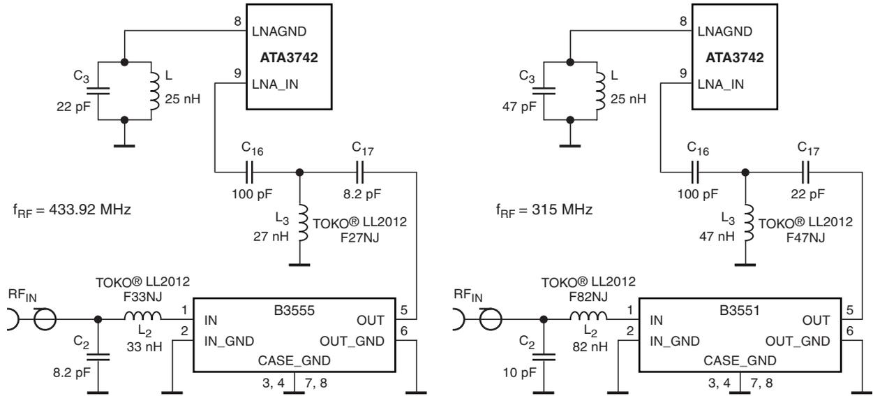
**Figure 3-3.** Input Matching Network Without SAW Filter
