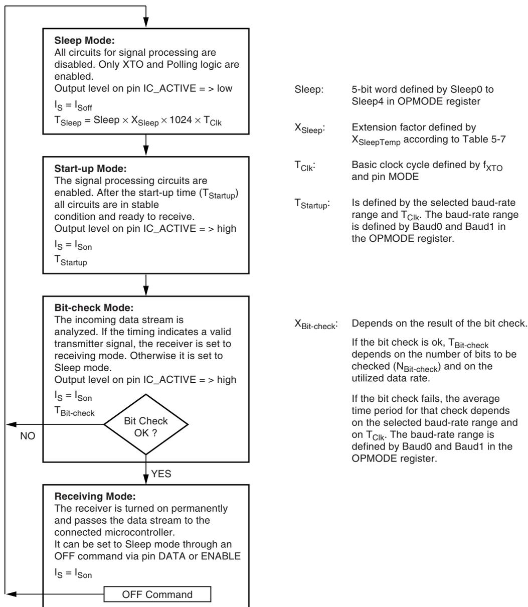
**Figure 5-4.** Timing Diagram for Complete Successful Bit Check
