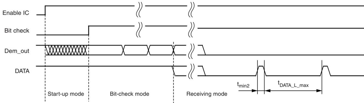
After the end of data transmission, the receiver remains active and random noise pulses appear at pin DATA. The edge-to-edge time period  $t_{ee}$  of the majority of these noise pulses is equal to or slightly higher than  $T_{DATA\_min}$ .
