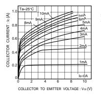
Fig.1 Ground emitter output characteristics
