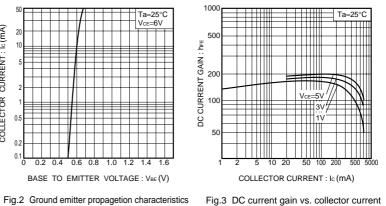
Fig.3 DC current gain vs. collector current
