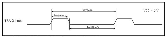
Figure 5.5 TRAIO Input Timing Diagram when Vcc = 5 V
