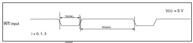
Figure 5.7 External Interrupt INTi Input Timing Diagram when Vcc = 5 V
