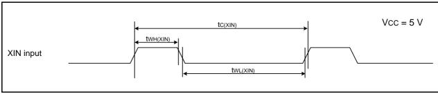
Figure 5.4 XIN Input Timing Diagram when Vcc = 5 V
