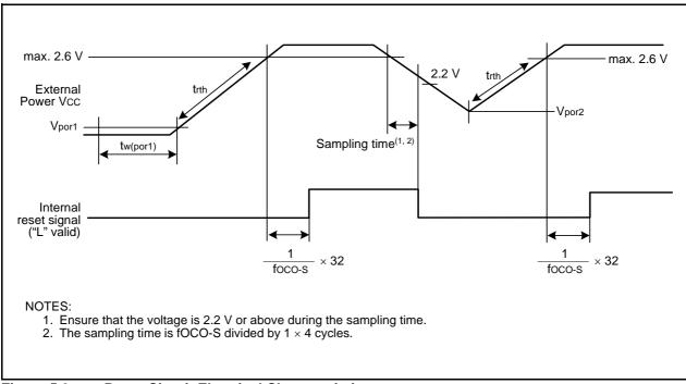
Figure 5.3 Reset Circuit Electrical Characteristics
