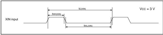
Figure 5.8 XIN Input Timing Diagram when Vcc = 3 V
