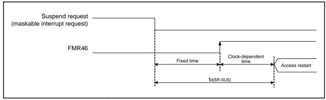
Figure 5.2 Time delay until Suspend
