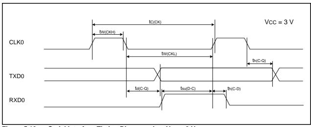
Figure 5.10 Serial Interface Timing Diagram when Vcc = 3 V
