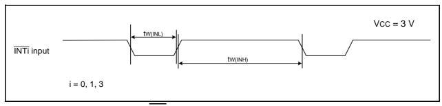
Figure 5.11 External Interrupt INTi Input Timing Diagram when Vcc = 3 V
