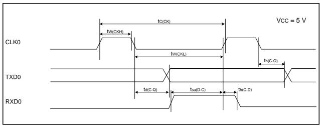
Figure 5.6 Serial Interface Timing Diagram when Vcc = 5 V
