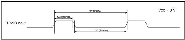
Figure 5.9 TRAIO Input Timing Diagram when Vcc = 3 V
