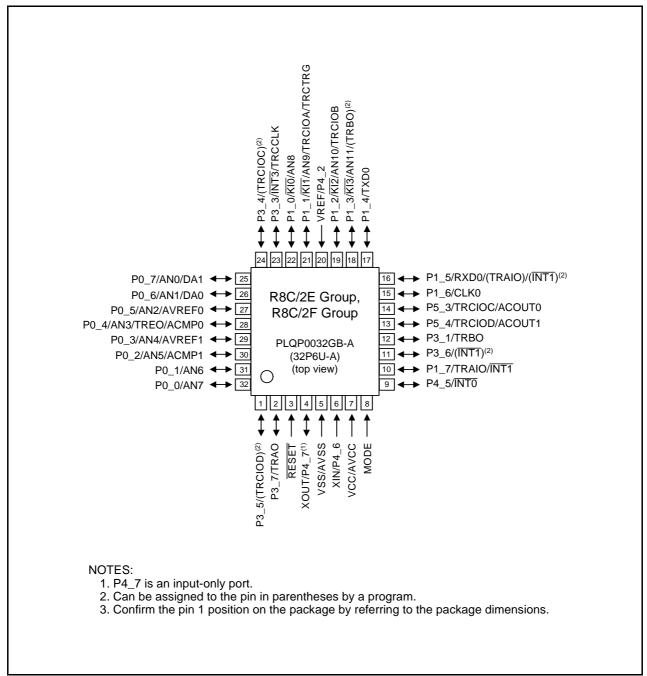
Figure 1.4 Pin Assignments (Top View)
