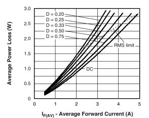
Fig. 6 - Forward Power Loss Characteristics
