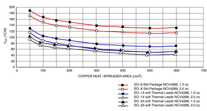
Figure 19. Junction-to-Ambient Thermal Resistance ( $\theta_{JA}$ ) vs. Heat Spreader Area
