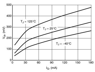
Figure 7. Drop Voltage V<sub>dr</sub> vs. Output Current I<sub>Q</sub>
