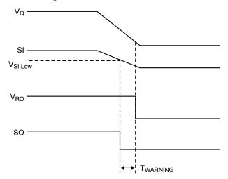
Figure 22. SO Warning Waveform Time Diagram
