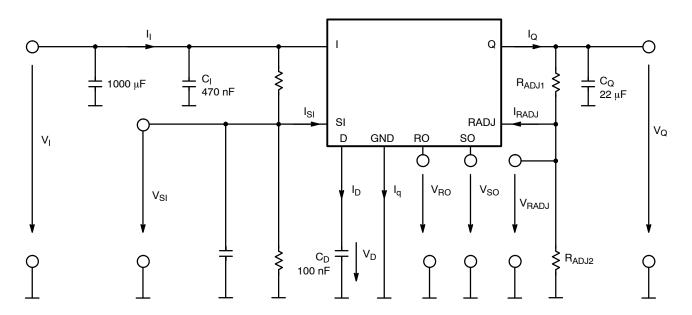
Figure 2. Measuring Circuit
