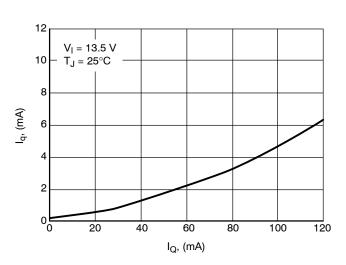
Figure 14. Current Consumption  $I_q$  vs. Output Current  $I_Q$
