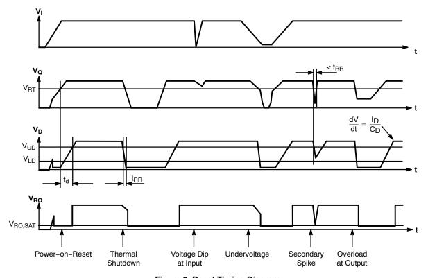
Figure 3. Reset Timing Diagram
