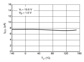
Figure 5. Charge Current  $I_{\text{D,C}}$  vs. Temperature  $T_{\text{J}}$
