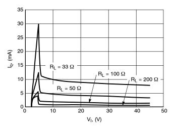
Figure 9. Current Consumption  $I_q$  vs. Input Voltage  $V_l$
