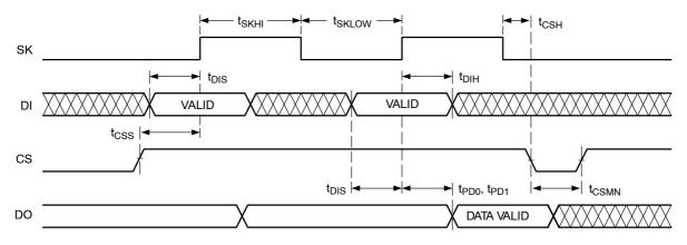
Figure 2. Synchronous Data Timing
