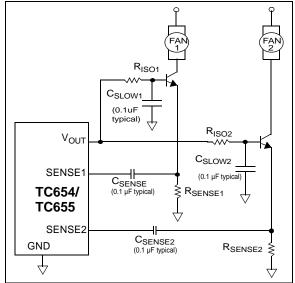
**FIGURE 7-11:** Transistor Drive with  $C_{SLOW}$  Capacitor.
