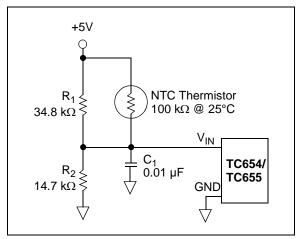
FIGURE 4-6: NTC Thermistor Sensor Network.
