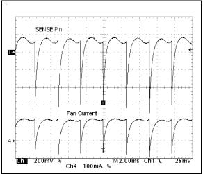
FIGURE 7-6: Typical Fan Current and Sense Pin Waveforms.
