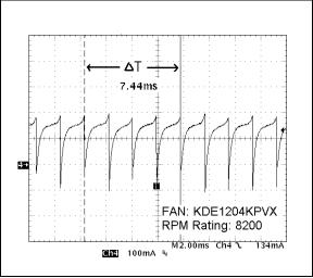
FIGURE 7-9: Four Current Pulses Per Revolution Fan.
