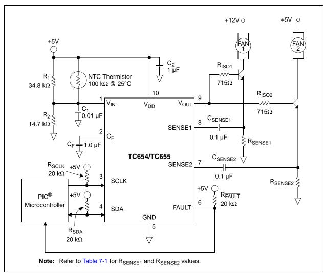
FIGURE 4-1: Typical Application Circuit.
