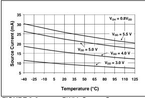
FIGURE 2-3: PWM, Source Current vs. Temperature.
