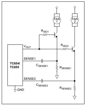
FIGURE 4-7: Fan Current Sensing.
