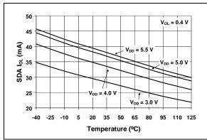
FIGURE 2-7: SDA I<sub>OL</sub> vs. Temperature.
