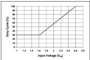
**FIGURE 4-5:** PWM Duty Cycle vs. V<sub>IN</sub> Voltage (Typical).
