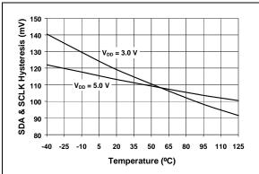
FIGURE 2-12: SDA, SCLK Hysteresis vs. Temperature.
