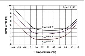
FIGURE 2-10: RPM %error vs. Temperature.
