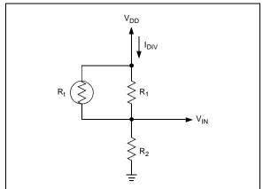
FIGURE 7-3: Temperature Sensing Circuit.
