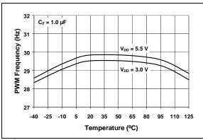
FIGURE 2-6: PWM Frequency vs. Temperature.
