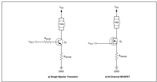
FIGURE 7-7: Output Drive Device Configurations.
