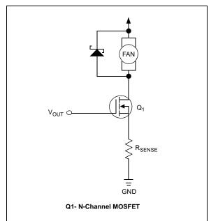
FIGURE 7-8: Clamp Diode For Fan Turn-Off.
