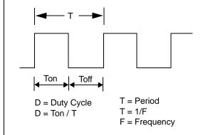
FIGURE 4-2: Duty Cycle Of A PWM Waveform.
