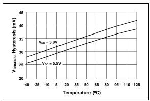
**FIGURE 2-11:** Sense Threshold (V<sub>THSENSE</sub>) Hysteresis vs. Temperature.
