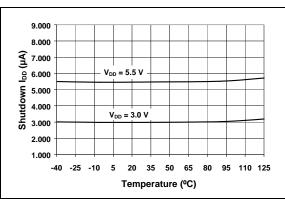
**FIGURE 2-2:** I<sub>DD</sub> Shutdown vs. Temperature.
