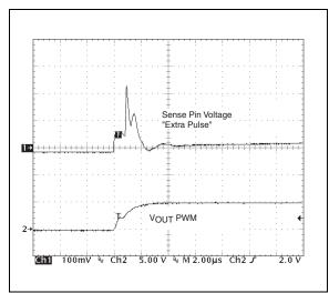
FIGURE 7-10: Extra Pulse at Sense Pin.
