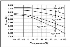
FIGURE 2-8: V<sub>CMAX</sub> vs. Temperature.
