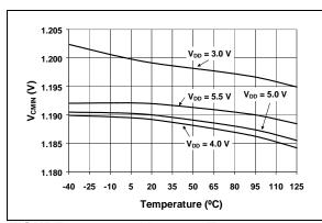
FIGURE 2-9: V<sub>CMIN</sub> vs. Temperature.
