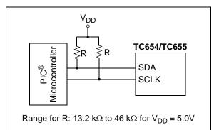
FIGURE 7-1: Pull-up Resistors On SMBus.
