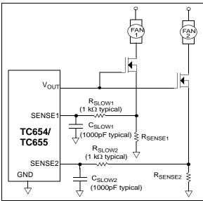
FIGURE 7-12: FET Drive with R<sub>SLOW</sub>/C<sub>SLOW</sub> Sense Scheme.
