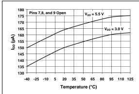
FIGURE 2-1: I<sub>DD</sub> vs. Temperature.
