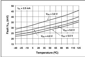
FIGURE 2-5: Fault V<sub>OL</sub> vs. Temperature.
