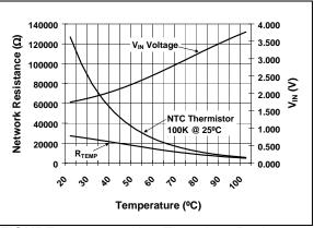
**FIGURE 7-4:** How Thermistor Resistance,  $V_{IN}$ , And  $R_{TEMP}$  Vary With Temperature.
