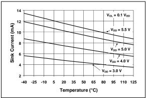
**FIGURE 2-4:** PWM, Sink Current vs. Temperature.
