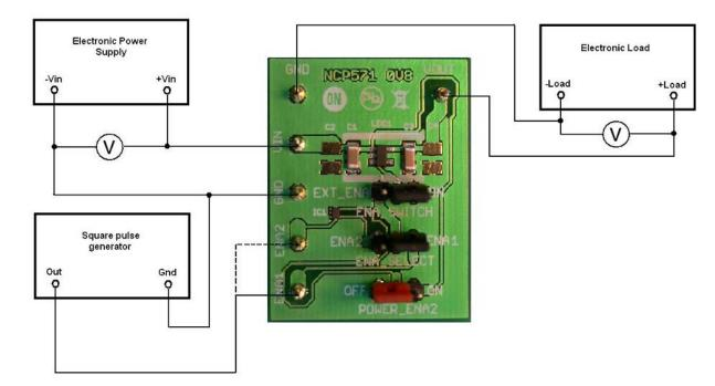
1. Enable pin connected to Vin
