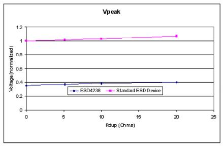
Figure 5. Normalized V<sub>Peak</sub> (8 kV IEC-61000 4-2 ESD Contact Strike) vs. Loading (RDUP)\*
