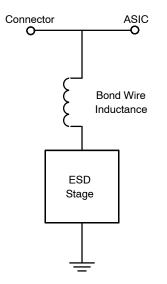
Figure 3. Standard ESD Protection Model
