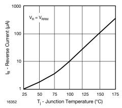
Fig. 4 - Reverse Current vs. Junction Temperature
