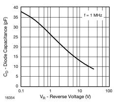
Fig. 6 - Diode Capacitance vs. Reverse Voltage
