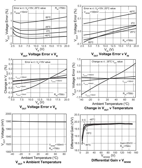
Test conditions unless otherwise stated:  $T_A$  = 25°C,  $V_B$  =  $V_{SENSE+}$  (via  $R_{SH}$ ) =15V,  $V_{SENSE}$  = 100mV  $R_G$  = 15k $\Omega$ .
