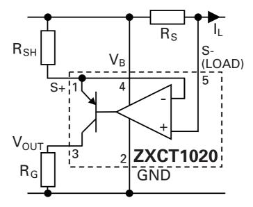
$R_{SH}$  sets the transconductance whereas  $R_{G}$  set the gain and results in an output voltage defined as:
