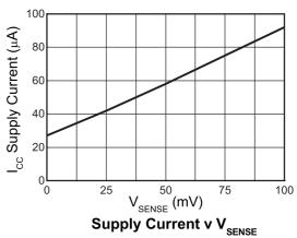
Test conditions unless otherwise stated:  $T_A$  = 25°C,  $V_B$  =  $V_{SENSE+}$  (via  $R_{SH}$ ) =15V,  $V_{SENSE}$  = 100mV Gain = 10,  $R_G$  = 15k $\Omega$ .
