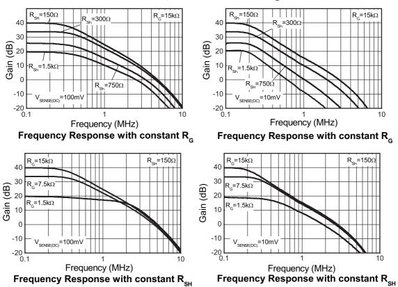
Test conditions unless otherwise stated:  $T_A = 25^{\circ}C$ , G=100,  $R_G = 15k$ ,  $V_B = V_{SENSE+}$  (via  $R_{SH}$ ),  $V_{SENSE} = 100 \text{mV}$ .
