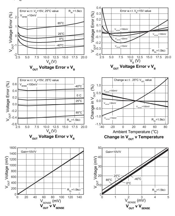
Test conditions unless otherwise stated:  $T_A = 25^{\circ}C$ ,  $V_B = V_{SENSE+}$  (via  $R_{SH}$ ) =15V,  $V_{SENSE} = 100 \text{mV}$  Gain = 20,  $R_G = 15 \text{k}\Omega$ .
