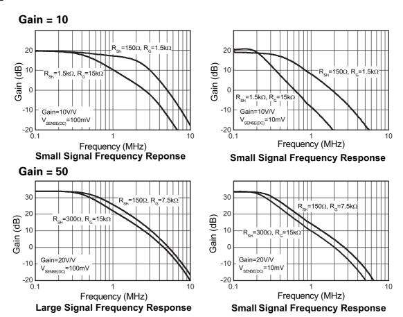
Test conditions unless otherwise stated:  $T_A$  = 25°C,  $R_G$ =15k,  $V_B$  =  $V_{SENSE+}$  (via  $R_{SH}$ ) =15V,  $V_{SENSE}$  = 100mV unless otherwise stated.
