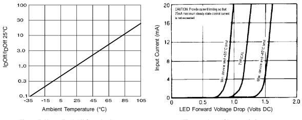
Figure 5. Normalized Off-State Leakage
