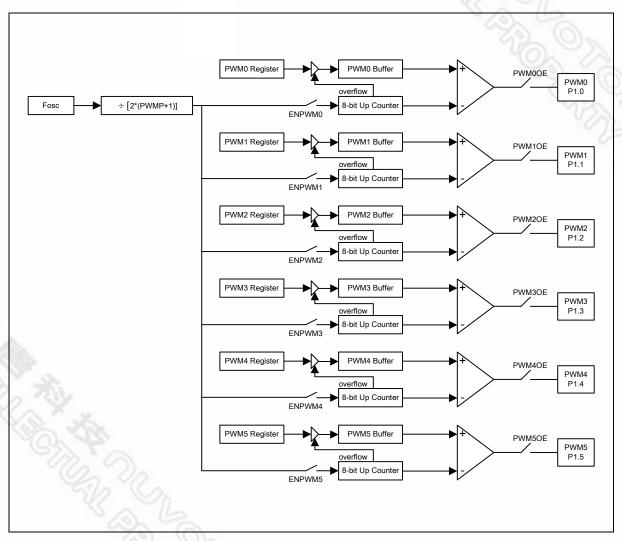
Figure 13-1 PWM block diagram
