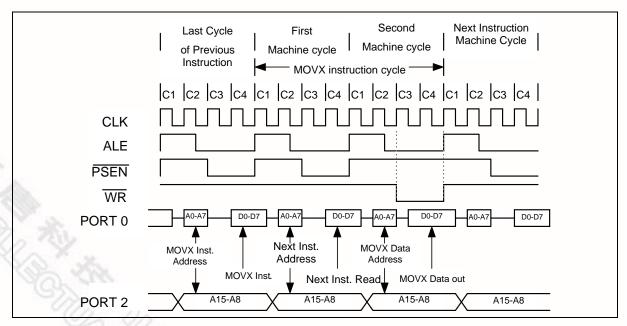
Figure 7-6 Data Memory Write with Stretch Value = 0
