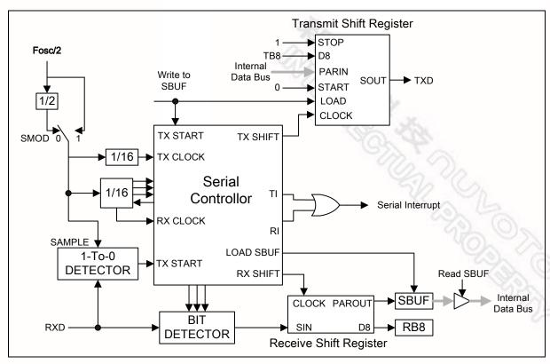
Figure 14-3 Serial Port Mode 2
