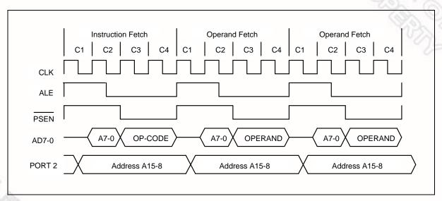
Figure 7-3 Three Cycle Instruction Timing
