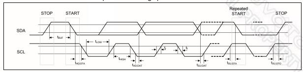
Figure 15-1 I2C Bus Timing
