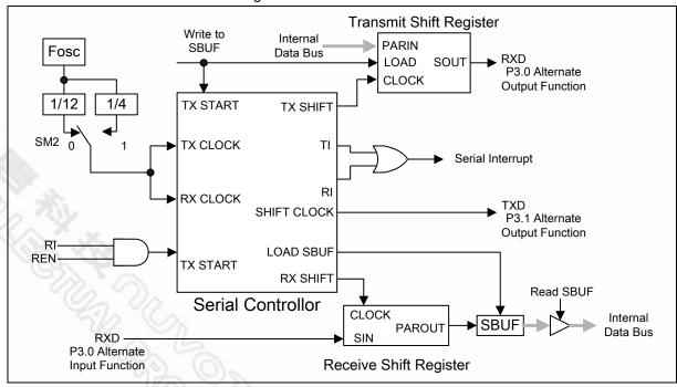
Figure 14-1 Serial Port Mode 0
