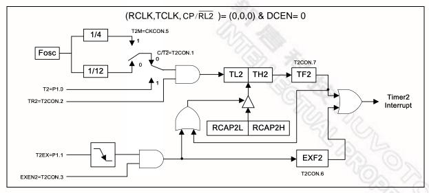
Figure 11-5 16-Bit Auto-reload Mode, Counting Up
