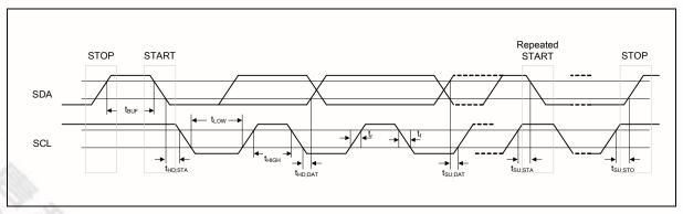
Figure 23-1 I2C Bus Timing
