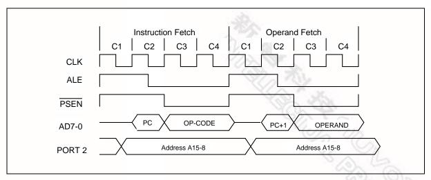
Figure 7-2 Two Cycle Instruction Timing
