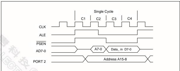
Figure 7-1 Single Cycle Instruction Timing
