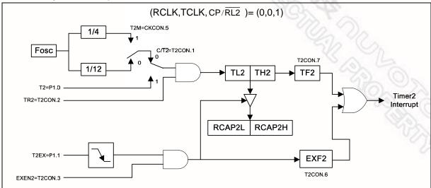
Figure 11-4 Timer2 16-Bit Capture Mode
