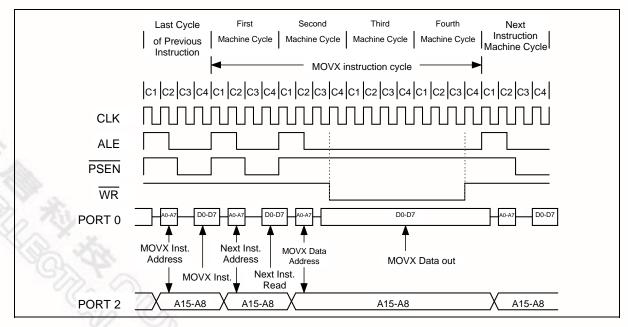
Figure 7-8 Data Memory Write with Stretch Value = 2
