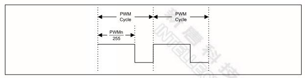
Figure 13-2 PWM Duty Ratio
