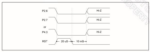
Figure 19-1 Timing of Entering Re-Boot Mode
