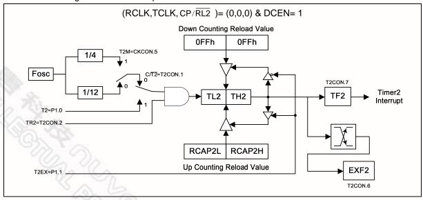
Figure 11-6 16-Bit Auto-reload Up/Down Counter
