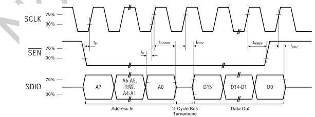
Figure 5. 3-Wire Control Interface Read Timing Parameters
