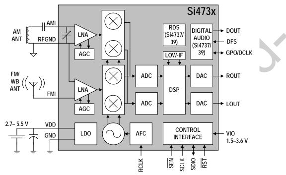
Figure 9. Functional Block Diagram
