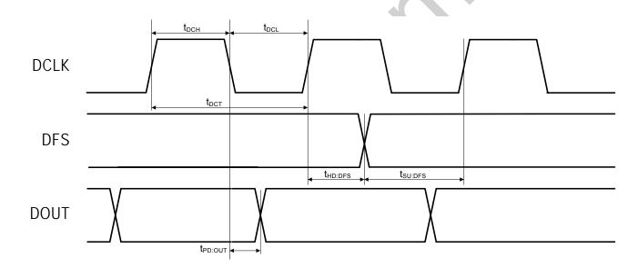
Figure 8. Digital Audio Interface Timing Parameters, I<sup>2</sup>S Mode
