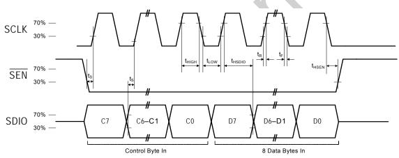
Figure 6. SPI Control Interface Write Timing Parameters
