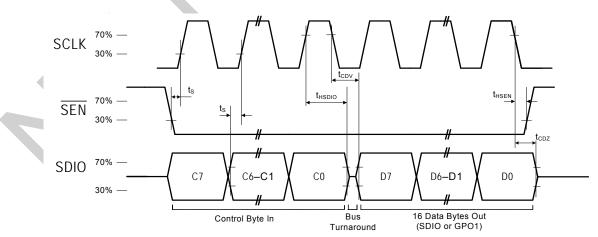
Figure 7. SPI Control Interface Read Timing Parameters
