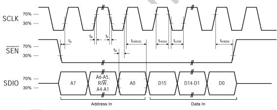
Figure 4. 3-Wire Control Interface Write Timing Parameters
