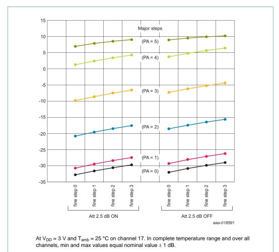
Fig 51. Typical control range output power
