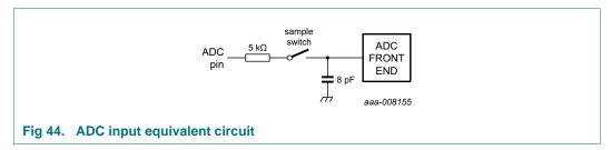
The ADC sampling period, input range and mode (single shot or continuous) are controlled through software.
