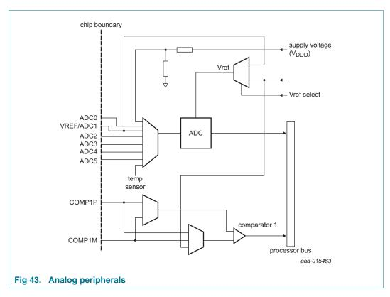
In order to provide good isolation from digital noise, the analog peripherals and radio are powered by the radio regulator, which is supplied from the analog supply  $V_{DDA}$  and referenced to analog ground  $V_{SSA}$ .
