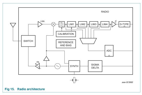
The radio comprises a low-IF receive path and a direct modulation transmit path, which converge at the TX/RX switch. The switch connects to the external single ended matching network, which consists of two inductors and a capacitor; this arrangement creates a 50  $\Omega$  port and removes the need for a balun. A 50  $\Omega$  single-ended antenna can be connected directly to this port.
