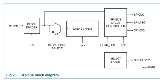
The SPI-bus employs a simple shift-register data transfer scheme. Data is clocked out of and into the active devices in a first-in, first-out fashion allowing SPI-bus devices to transmit and receive data simultaneously. Master-Out-Slave-In or Master-In-Slave-Out data transfer is relative to the clock signal SPICLK generated by the JN517x.
