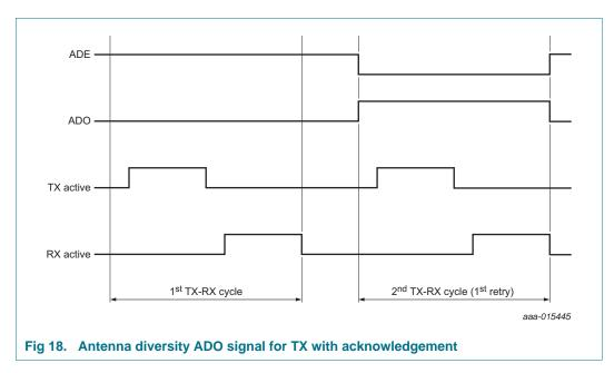
If two DIO pins cannot be spared, one of the signals (ADE or ADO) from the JN517x can be used and its complement can be generated using an inverter on the PCB.
