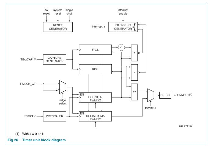
The clock source for the Timer0/Timer1 unit is fed from the system clock, selected as 16 MHz or 32 MHz. This clock passes to a 5-bit prescaler where a value of 0 leaves the clock unmodified and other values divide it by 2<sup>prescale value</sup>. For example, a prescale value of 2 applied to the 16 MHz system clock source results in a timer clock of 4 MHz.
