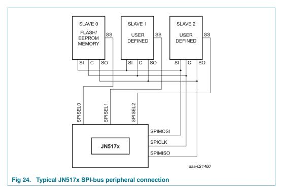
The data transfer rate on the SPI-bus is determined by the SPICLK signal. The JN517x supports transfers at data rates from 16 MHz to 125 kHz selected by a clock divider. Both SPICLK clock phase and polarity are configurable. The clock phase determines which edge of SPICLK is used by the JN517x to present new data on the SPIMOSI line; the opposite edge will be used to read data from the SPIMISO line. The interface should be configured appropriately for the SPI-bus slave being accessed.
