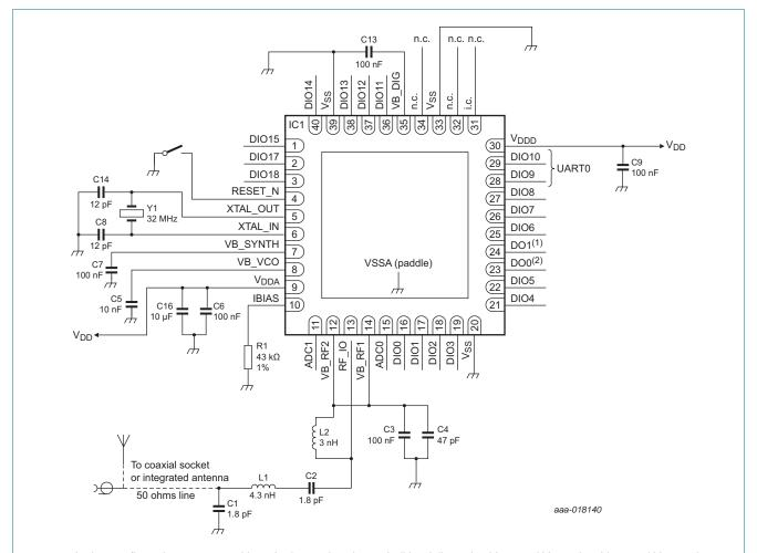
In that configuration, an external low ohmic supply voltage shall be delivered to  $V_{DDA}$  and  $V_{DDD}$  pins.  $V_{DDA}$  and  $V_{DDD}$  voltages shall be minimum 2.0 V and maximum 3.6 V, the supply source shall be connected directly to the device pins without any serial resistor.
