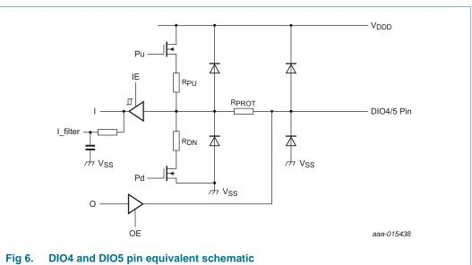
In reset, the digital peripherals are all OFF and the DIO pins are set as high-impedance inputs. During sleep and deep sleep, the DIO pins retain both their input/output state and output level that was set as sleep commences. If the DIO pins were enabled as inputs and the interrupts were enabled, then these pins may be used to wake up the JN517x from sleep or deep sleep.
