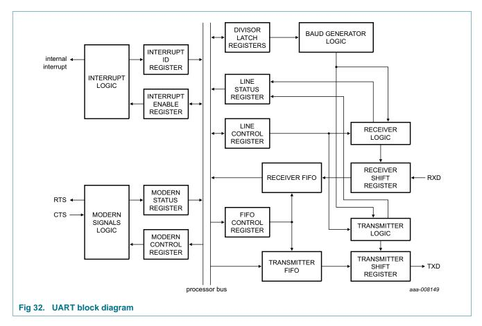
The serial interfaces contain programmable fields that can be used to set number of data bits (5, 6, 7 or 8), even, odd, set-at-1, set-at-0 or no-parity detection and generation of single or multiple stop bit (for 5-bit data, multiple is 1.5 stop bits; for 6 data bits or 7 data bits or 8 data bits, multiple is 2 bits).
