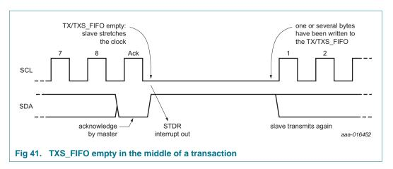
A transaction is aborted only when the master does not acknowledge a data byte, after which the slave releases the data line. A STOP or a RESTART is then issued by the master.
