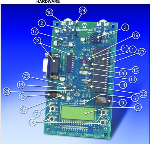
FIGURE 1-1: LOW POWER SOLUTIONS DEMONSTRATION BOARD HARDWARE
