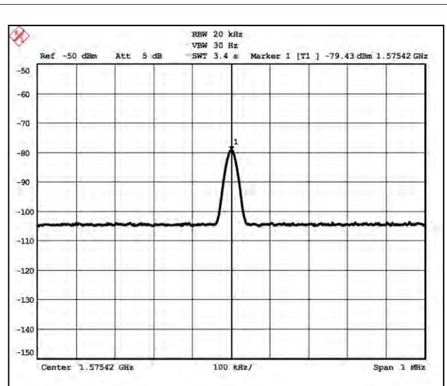
Fig 9. FE output IM3 level at 1575.42 MHz
