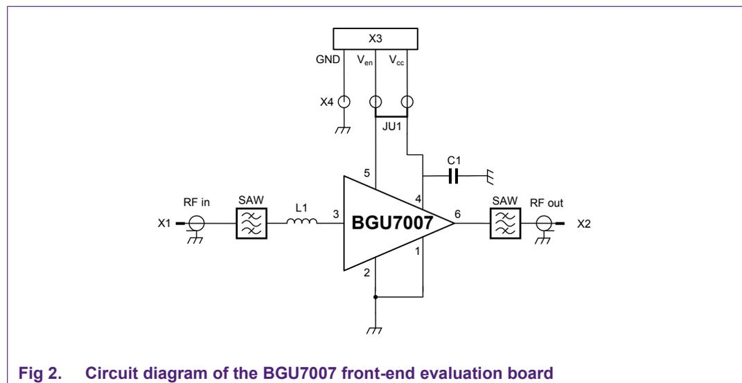
Fig 2. Circuit diagram of the BGU7007 front-end evaluation board
