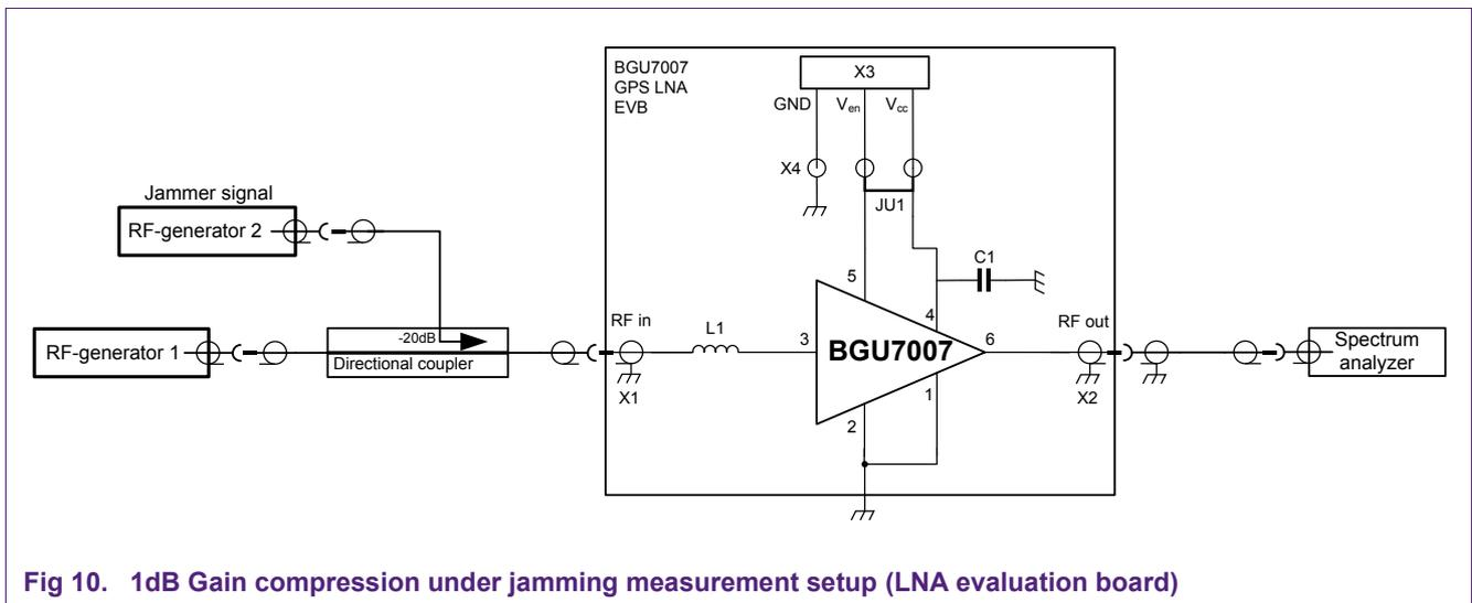
Fig 10. 1dB Gain compression under jamming measurement setup (LNA evaluation board)
