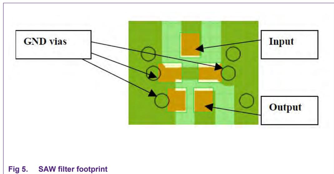
Fig 5. SAW filter footprint
