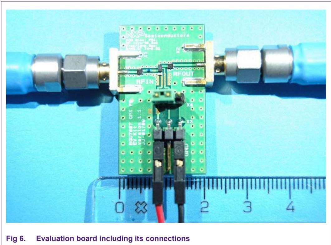
Fig 6. Evaluation board including its connections
