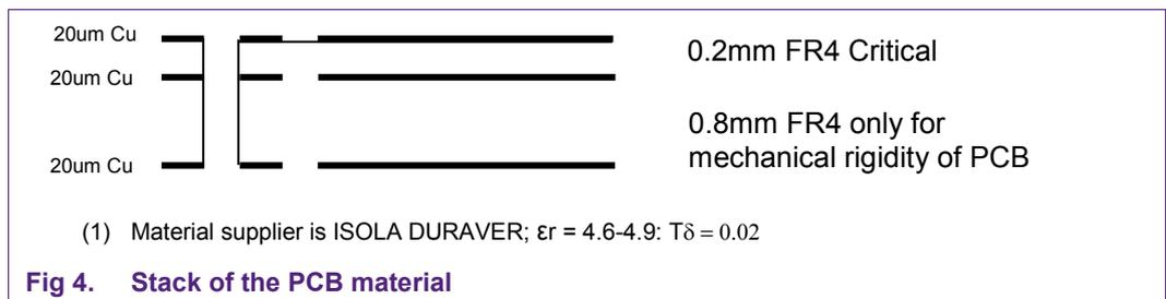
Fig 4. Stack of the PCB material
