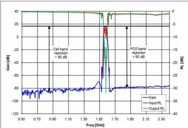
Fig 16. Typical S-parameter plot at Vcc = 1.8 V
