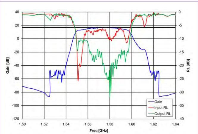
Fig 17. Typical pass band response at Vcc = 1.8 V
