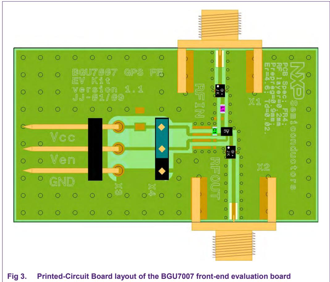
Fig 3. Printed-Circuit Board layout of the BGU7007 front-end evaluation board
