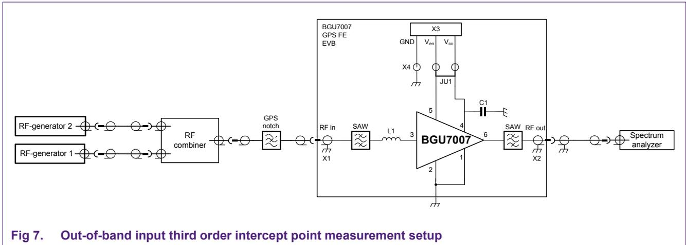
Fig 7. Out-of-band input third order intercept point measurement setup
