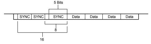
Figure 9. Detecting 5- or 7-Bit Synchronous Characters
