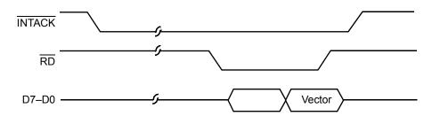
Figure 22. Interrupt Acknowledge Cycle Timing (Z85230/L)
