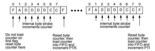
Figure 16. SDLC Byte Counting Detail
