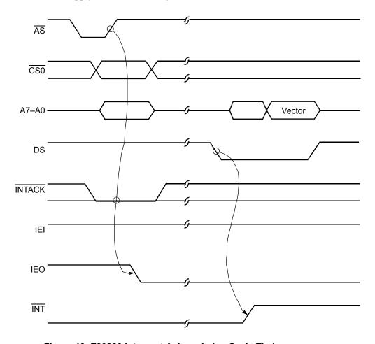
Figure 19. Z80230 Interrupt Acknowledge Cycle Timing
