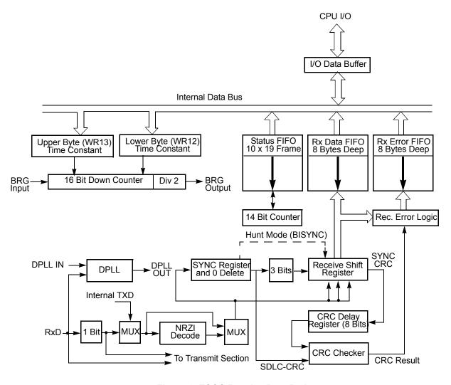
Figure 6. ESCC Receive Data Path
