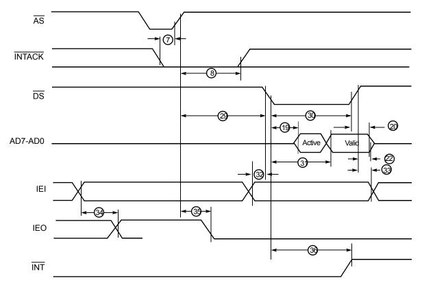
Figure 25. Z80230 Interrupt Acknowledge Timing Diagram
