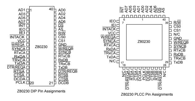
Figure 4. Z80230 Pin Assignments
