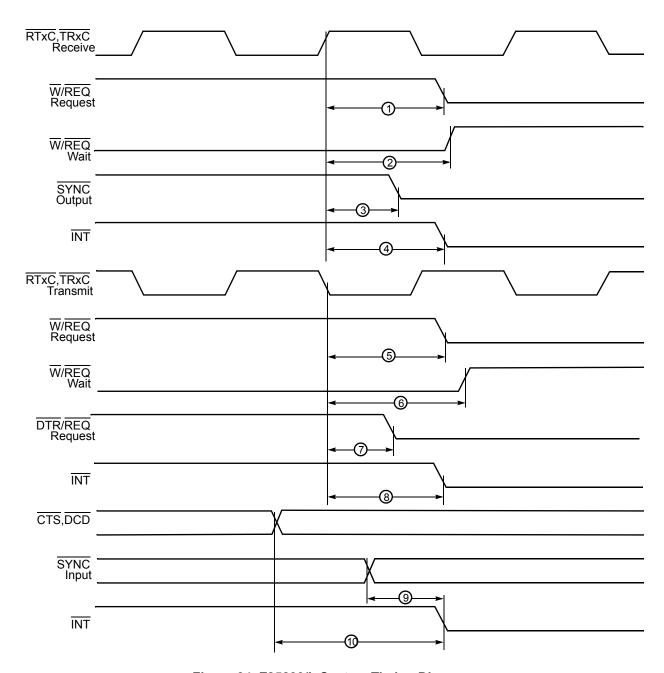
Figure 34. Z85230/L System Timing Diagram
