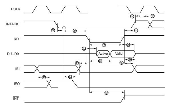
Figure 31. Z85230/L Interrupt Acknowledge Timing Diagram
