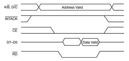
Figure 20. Read Cycle Timing (Z85230/L)
