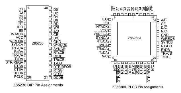
Figure 3. Z85230/L Pin Assignments
