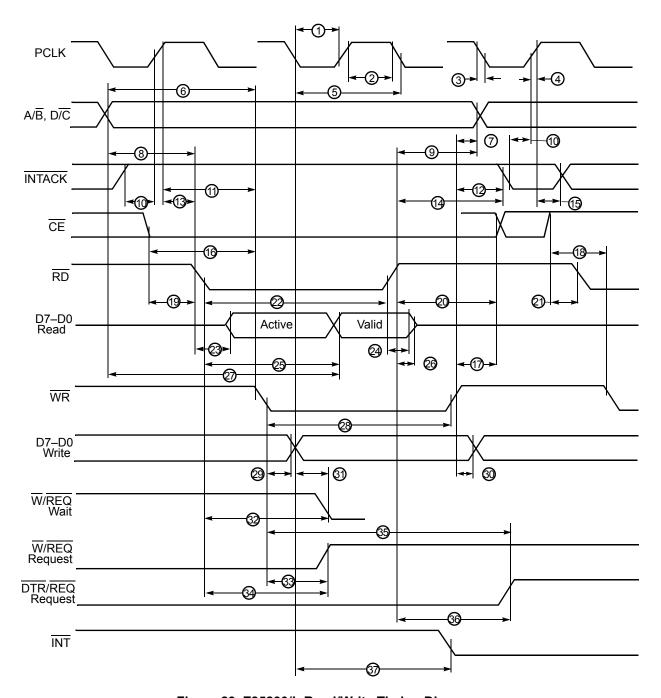
Figure 29. Z85230/L Read/Write Timing Diagram
