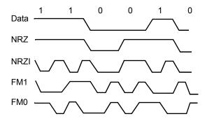
Figure 11. Data Encoding Methods
