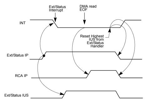
Resetting highest IUS from lower priority interrupt clears the EOF (RCA) interrupt.
