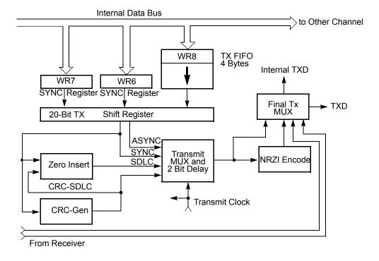
Figure 5. ESCC Transmit Data Path
