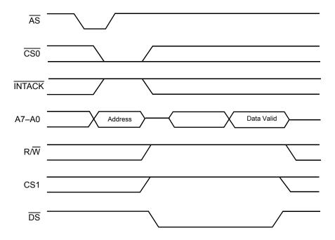
Figure 18. Z80230 Read Cycle Timing
