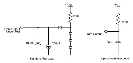
Figure 23. Standard and Open-Drain Test Loads
