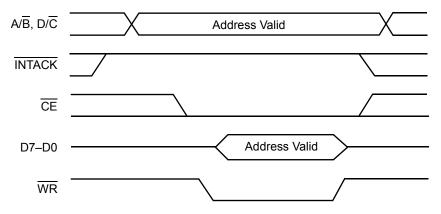
Figure 21. Write Cycle Timing (Z85230/L)
