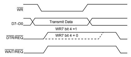
Figure 12. DMA Request on Transmit Deactivation Timing
