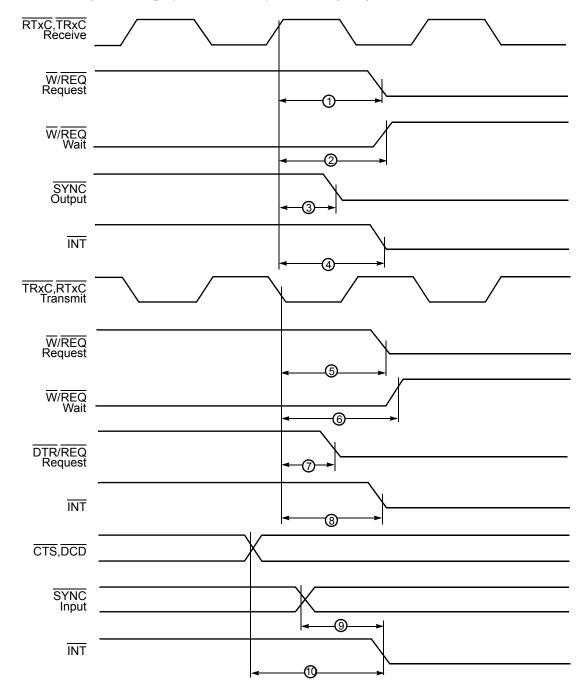
Figure 28. Z80230 System Timing Diagram
