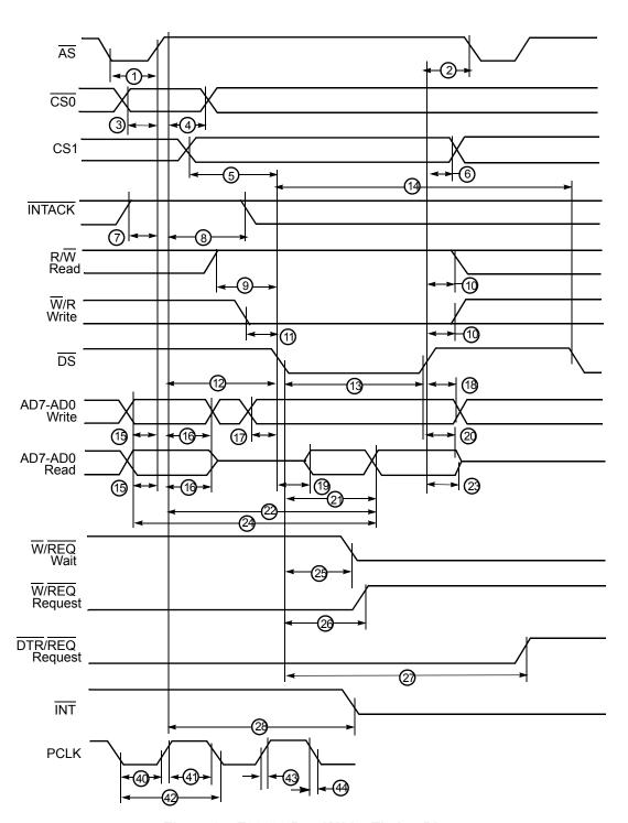
Figure 24. Z80230 Read/Write Timing Diagram
