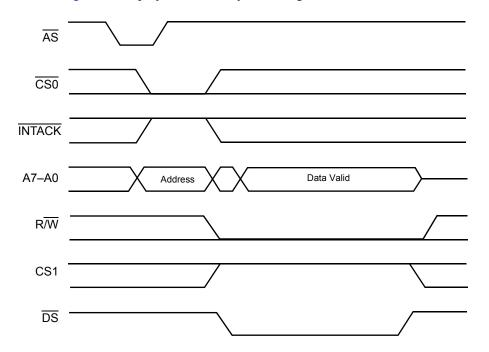
Figure 17. Z80230 Write Cycle Timing
