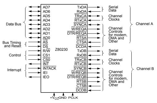
Figure 2. Z80230 Pin Functions
