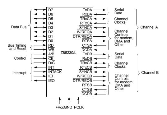
Figure 1. Z85230/L Pin Functions
