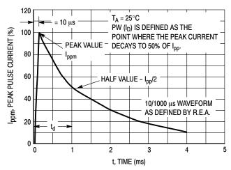
Figure 1. Pulse Rating Curve
