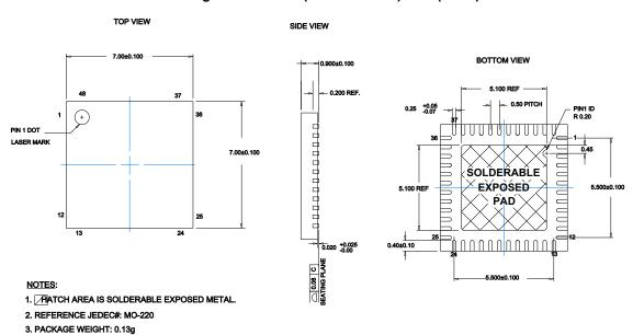
Figure 15. 48-Pin (7 × 7 × 1.0 mm) QFN (Sawn)
