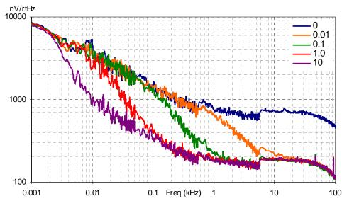
Figure 11. Typical AGND Noise with P2[4] Bypass
