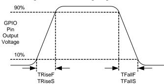
Figure 10. GPIO Timing Diagram
