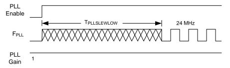
Figure 9. External Crystal Oscillator Startup Timing Diagram
