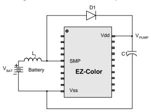
Figure 6. Basic Switch Mode Pump Circuit
