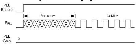
Figure 8. PLL Lock for Low Gain Setting Timing Diagram
