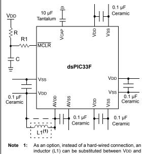
Note 1: As an option, instead of a hard-wired connection, an inductor (L1) can be substituted between VDD and AVDD to improve ADC noise rejection. The inductor impedance should be less than 1Ω and the inductor capacity greater than 10 mA.
