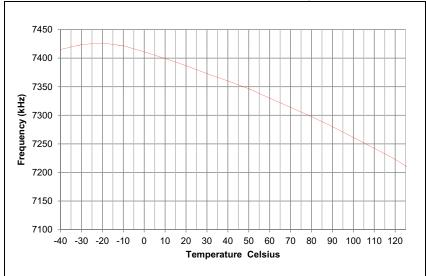
FIGURE 26-14: TYPICAL LPRC FREQUENCY @ VDD = 3.3V
