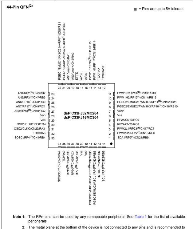
2: The metal plane at the bottom of the device is not connected to any pins and is recommended to be connected to Vss externally.
