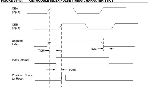
FIGURE 24-13: **QEI MODULE INDEX PULSE TIMING CHARACTERISTICS**
