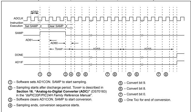
FIGURE 24-28: ADC CONVERSION (10-BIT MODE) TIMING CHARACTERISTICS (CHPS<1:0> = 01, SIMSAM = 0, ASAM = 1, SSRC<2:0> = 111, SAMC<4:0> = 00001)
