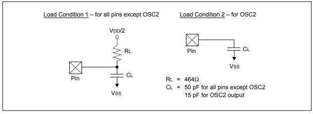
TABLE 24-15: CAPACITIVE LOADING REQUIREMENTS ON OUTPUT PINS
