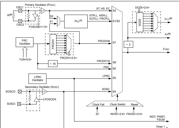
FIGURE 8-1: dsPIC33FJ32MC202/204 and dsPIC33FJ16MC304 OSCILLATOR SYSTEM DIAGRAM
