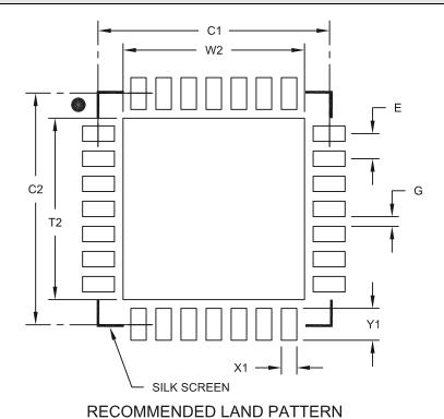
Units **MILLIMETERS** Dimension Limits MIN MOM MAX 0.65 BSC Contact Pitch Ε Optional Center Pad Width W2 4.70 4.70 Optional Center Pad Length T2 Contact Pad Spacing 6.00 C1 Contact Pad Spacing C2 6.00 Contact Pad Width (X28) X1 0.40 Contact Pad Length (X28) <u>Y1</u> 0.85 Distance Between Pads G 0.25
