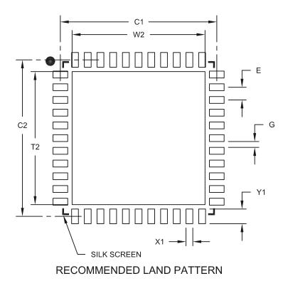
Units MILLIMETERS **Dimension Limits** MIN NOM MAX Contact Pitch Ε 0.65 BSC Optional Center Pad Width W2 6.80 Optional Center Pad Length T2 6.80 C1 8.00 Contact Pad Spacing C2 Contact Pad Spacing 8.00 Contact Pad Width (X44) X1 0.35 <u>Y1</u> 0.80 Contact Pad Length (X44) 0.25 Distance Between Pads G
