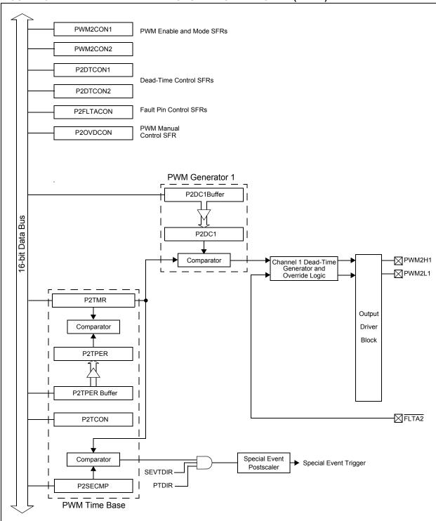
FIGURE 15-2: 2-CHANNEL PWM MODULE BLOCK DIAGRAM (PWM2)
