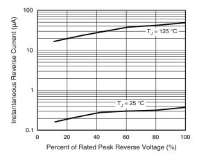
Fig. 4 - Typical Reverse Characteristics
