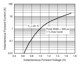
Fig. 3 - Typical Instantaneous Forward Characteristics
