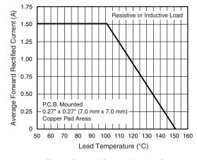
Fig. 1 - Forward Current Derating Curve
