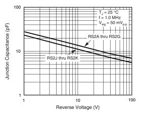
Fig. 5 - Typical Junction Capacitance
