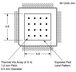
Figure 8. Recommended Thermal Land Pattern
