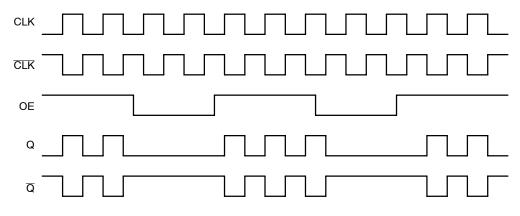
Figure 7. Output Enable (OE) Timing Diagram
