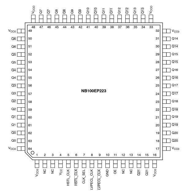
All V<sub>CC</sub>, V<sub>CCO</sub>, and GND pins must be externally connected to appropriate Power Supply to guarantee proper operation ( $V_{CC} \neq V_{CCO}$ ). The thermally conductive exposed pad on package bottom (see package case drawing) is electrically connected to GND internally.
